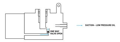
SV Now connect the bottom of the piston to the outlet.
